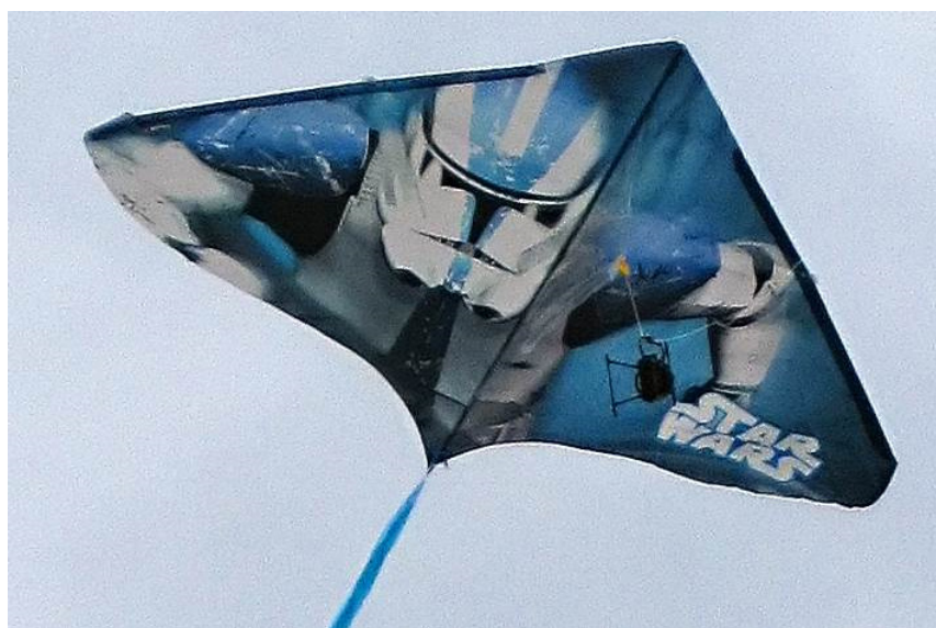
Figure 6. Kite hoisting a rotorless quadrotor-camera (a “nullicopter”), while capturing fig. 7.
